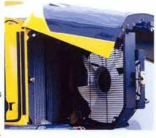
The radiator, air-to-air cooler and oil cooler are mounted side-by-side for more efficient cooling and easy cleaning. A fully-opening, gas spring assisted rear grill gives the operator excellent access to the swing-out fan and coolers.
