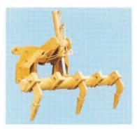
Rear-mounted ripper: Tool bar type. With hydraulically controlled raise and lower functions, this ripper can be used to dig out rocks or hard ground not removable by a scarifier.
