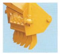
Scarifier: This attachment digs up hard ground, like asphalt, old pavement and frozen surfaces, which are not removable by the blade. The number of teeth can be changed according to ground hardness.
